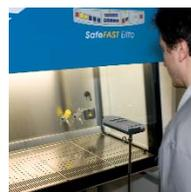
Each Faster vertical and horizontal laminar flow cabinet is tested in accordance to ISO 14644-1 and EN 61010:2001 Standards and released with FAT certificate of the tests performed.
